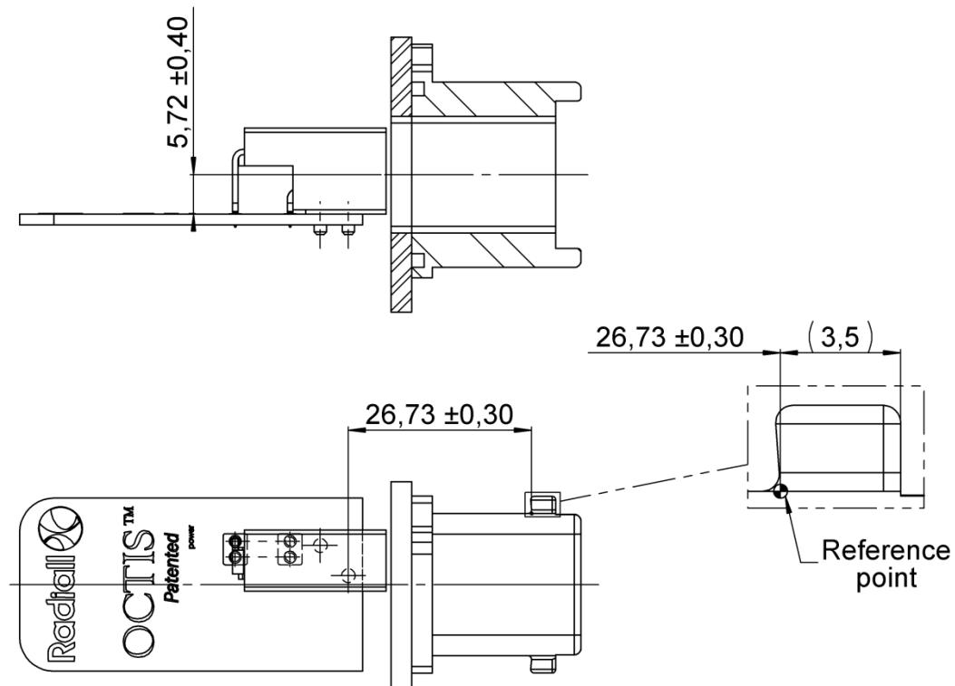
FOOT/PRINT (General tolerance for PCB  $\pm 0.1$  mm)
