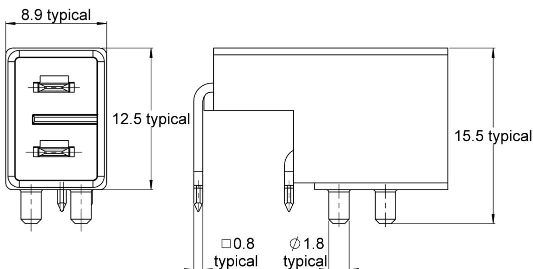
All dimensions are in mm. Unmarked tolerance is  $\pm 0.3$ mm
