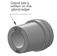
\*Cable diameter under the gland. If the cable has a sleeve, the diameter over the sleeve should be considered The tolerances of ΦD should be taken into account to make sure it is always within the specified range
