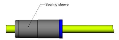
2- Strip the outer jacket and add the heat shrinkable sleeve ASNE0718-03 as illustrated
